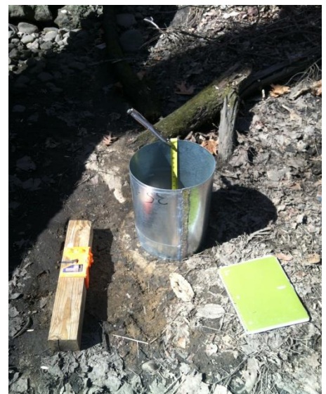
Figure 5: Photograph of the infiltrimeter test in the field
