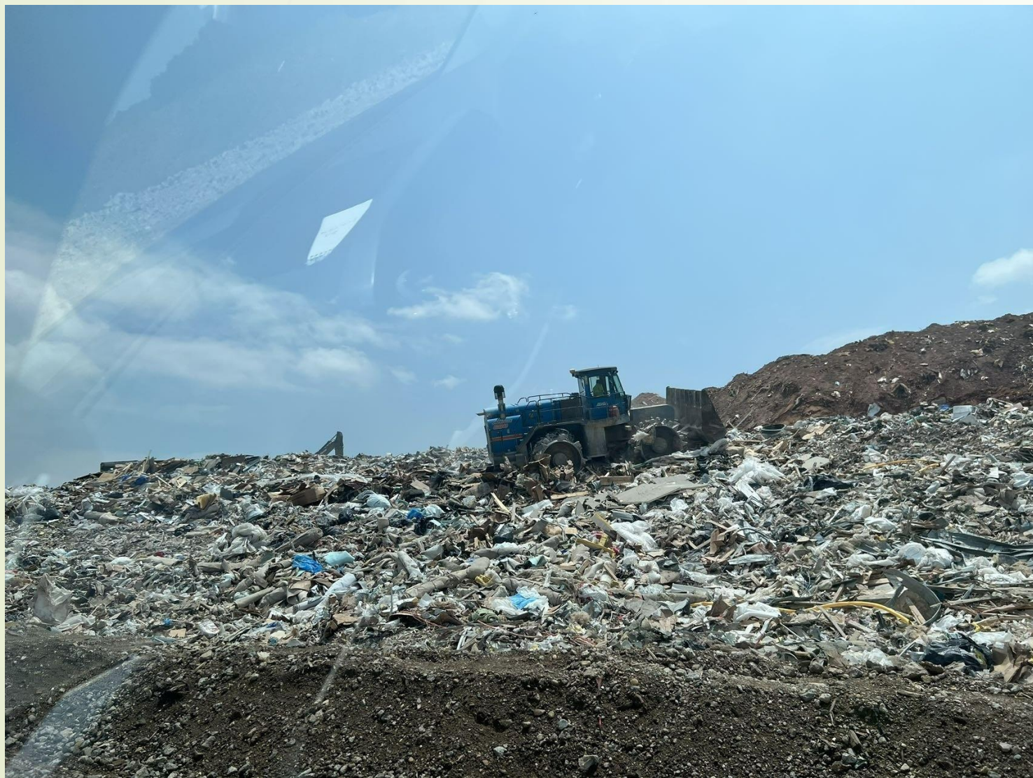
Landfilling area in Westphalia. This part has been filled up to a really high spot already, and there's the vehicle keep crushing on the waste residues to push them into more dense pieces.
