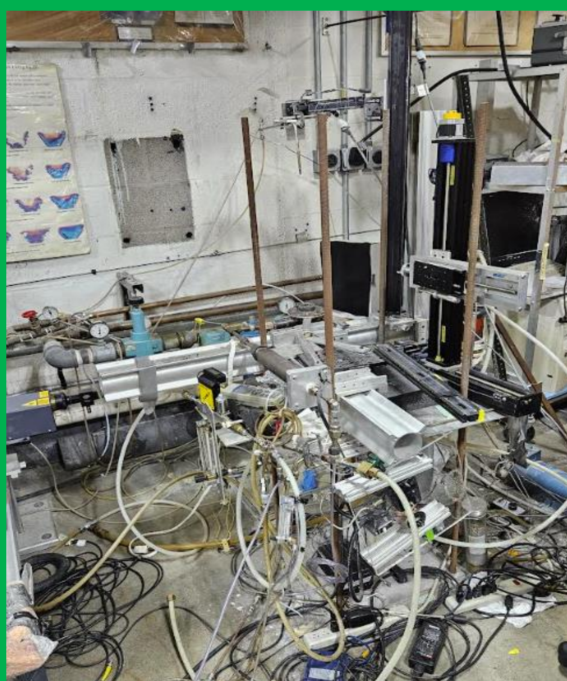
A picture of the combustor in the lab. The fuel lines connected to tanks sitting around the room. Fuels included hydrogen, methane, and propane, among others.
