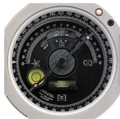
Figure 10 – Face of a Brunton Transit. Note the inner and outer scales. (Brunton, 2006)
