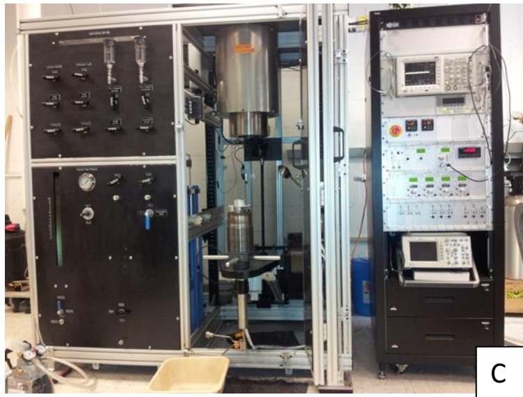
Figure C: Triaxial deformation apparatus: AutoLab 1500
