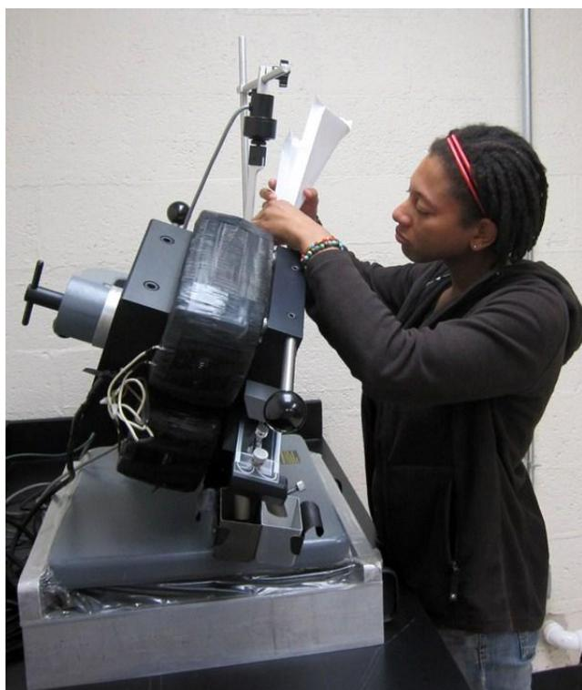
Fig. 5: Frantz magnetic barrier separator located in the Chemistry Building.
