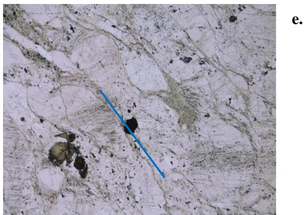
Figure 12: Photomicrographs of formations sampled: a) Mather Gorge Fm., b) Prettyboy Schist, c) E. Marburg Fm., d) W. Marburg Fm., e) Sams Creek Fm. All taken at 5x (2.7mm field of view), in plain polarized light. Blue lines indicate approximate orientation of foliation.
