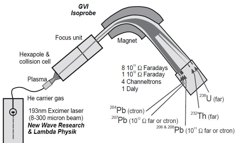
Fig. 6: LA-MC-ICP-MS at Arizona LaserChron Center in Tucson, AZ. Figure from Gehrels et al., 2006.
