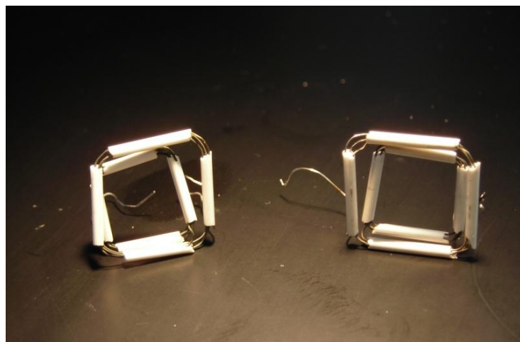
Figure 3. Heater with 4-hole alumina tubing and nichrome wire wound through each hole. Each heater is an approximate square with sides 20mm in length
