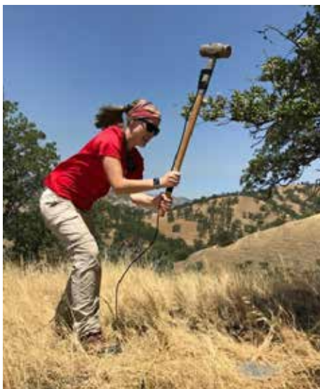
Rebecca Butcher is swinging a sledgehammer to generate active seismic source for a shallow seismic refraction survey in Williams, California.
